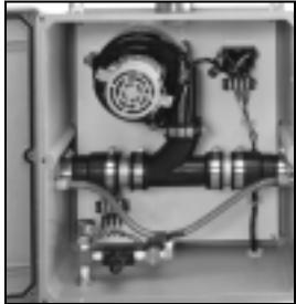
Sentinel II power heads can be controlled individually with nothing more complex than a toggle valve. Or you can get more automated, using solenoid valves on each low pressure feed line to turn heads on and off as needed.
