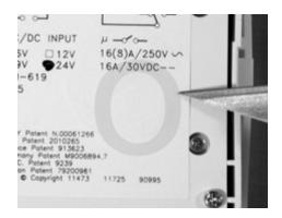
Remove the label, or cut along the outline of the cover with a sharp knife. Twist the cover to release. Replace with 3V CR2032 battery.
