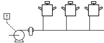
*Pressurized liquid source, such as the house water supply, feeding a zone of foggers. Solenoid valve is controlled by repeat cycle timer.*
